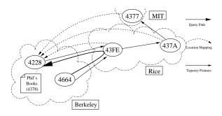
Figure 3: Route to object example, with local areas shown. A possible grouping of nodes from Figure 2 into local areas.
