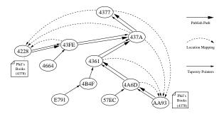
Figure 1: *Tapestry object publish example*. Two copies of an object (4378) are published to their root node at 4377. Publish messages are routed to root, depositing a location pointer for the object at each hop encountered along the way. Only relevant Tapestry pointers are shown.
