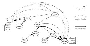
Figure 2: *Tapestry route to object example*. Several nodes send messages to object 4378 from different points in the network. The messages route towards the root node of 4378. When they intersect the publish path, they follow the location pointer to the nearest copy of the object.
