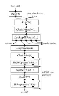
FIGURE 5—A portion of the IP router configuration.
