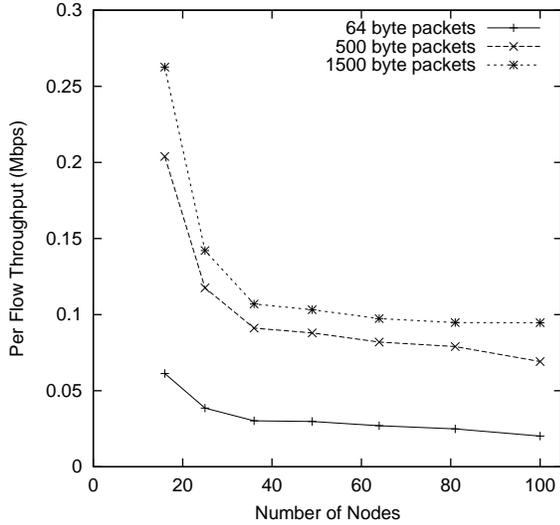
**Figure 8:** Average per flow throughput in square lattice networks with horizontal data streams only, as a function of network size. There are as many parallel chains as there are nodes per chain. The X axis value is the total number of nodes. Each node is separated from its four neighbors by 200 meters.
