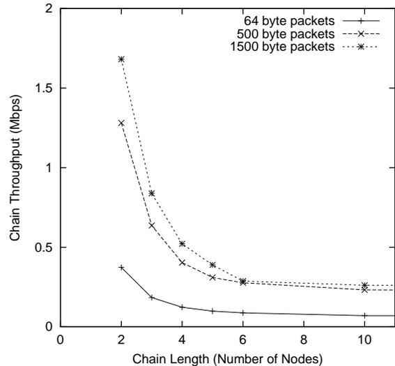
**Figure 3: Throughput achieved along a chain of nodes, as a function of the chain length. The nodes are 200 meters apart. The first node originates packets as fast as 802.11 allows, to be forwarded along the chain to the last node. The throughputs for chains of 20 and 50 nodes are the same as for 10 nodes.**
