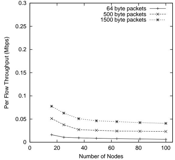
**Figure 9:** Average per flow throughput in square lattice networks with both horizontal and vertical data streams. This configuration has twice as many chains of traffic sharing the same network as Figure 8, which explains most of the difference between the two results.
