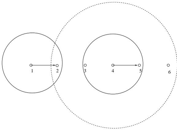
**Figure 2: MAC interference among a chain of nodes. The solid-line circle denotes a node's valid transmission range. The dotted-line circle denotes a node's interference range. Node 4's transmission will corrupt node 1's transmissions at node 2.**
