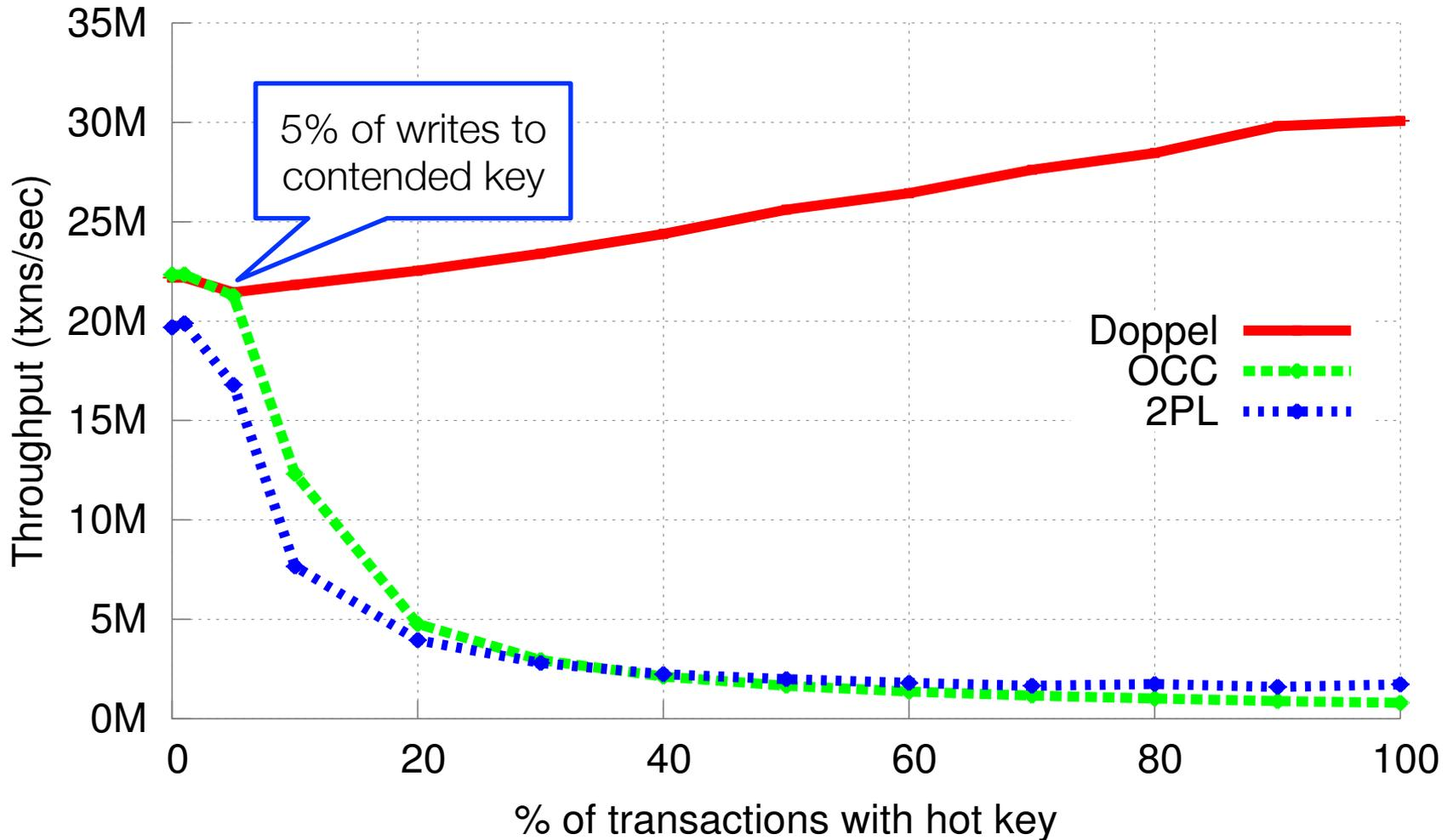
20 cores, 1M 16 byte keys, transaction: ADD(x,1) on different keys
