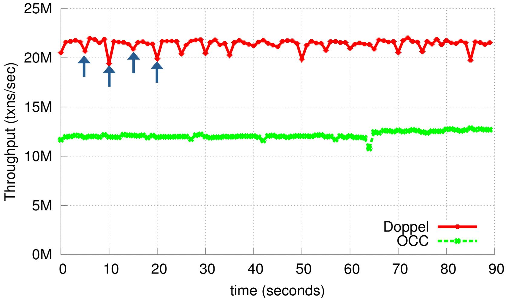
20 cores, 1M 16 byte keys, transaction: ADD(x,1) 10% on same key
