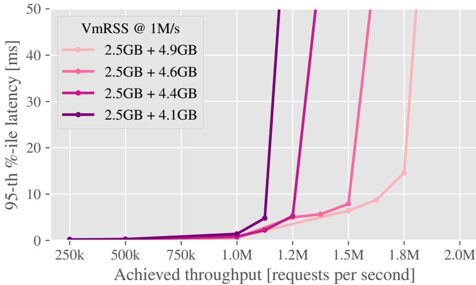
Figure 6.7.: Achieved throughput vs 95th percentile request latency in vote with increasingly aggressive eviction. Offered load increases along the points on each line. A near-vertical line indicates that the system no longer keeps up with offered load.
