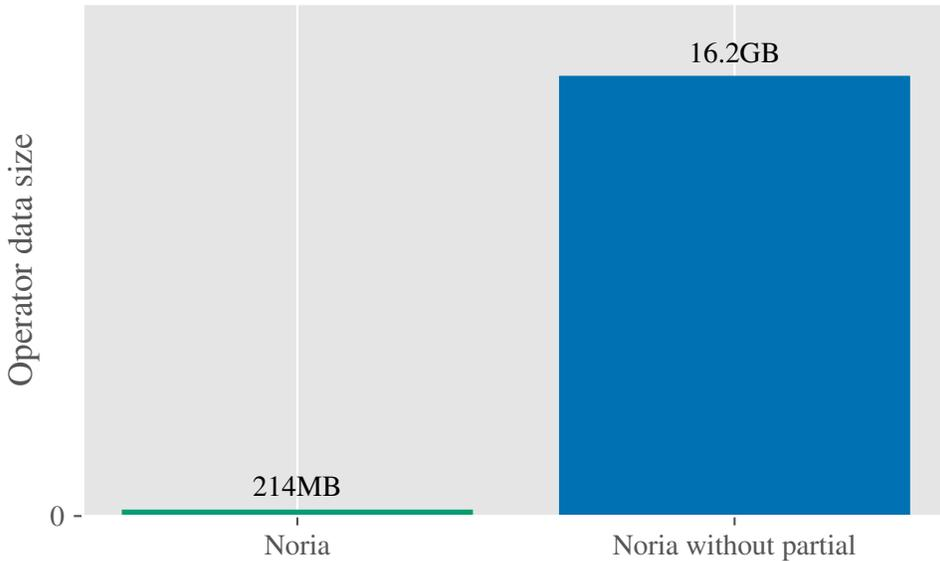
Figure 6.3.: Estimated operator state data size two minutes into the Lobsters benchmark at 4.6k pages per second. The value indicated includes only the sum total size of rows in each operator’s state, not data structure overheads, indices over the data, or other memory allocations. Base tables are not included.
