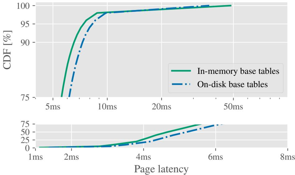
Figure 6.6.: CDF of sojourn latency across all Lobsters pages at 1.5k pages per second with base tables in memory and on disk. The figure depicts steady-state operation—the benchmark has been allowed to run for two minutes before the latency is measured.
