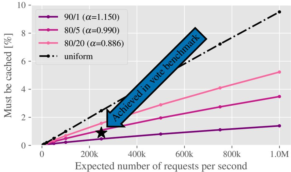
Figure 6.10.: Probabilistic model of the fraction of 10M keys that are accessed over the course of one second as throughput increases. Each line shows a different amount of skew. Skew (X/Y) denotes that X% of requests come from Y% of keys. More keys pushes the curve down.
