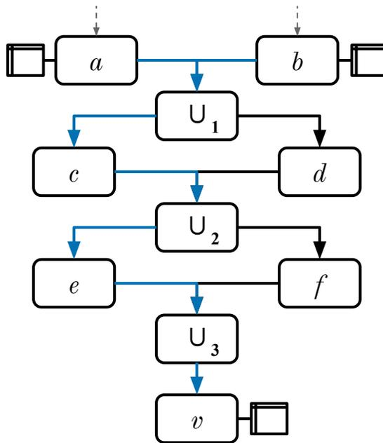
Figure 4.1.: Chained unions. Only nodes  $a$ ,  $b$ , and  $v$  hold state. Highlighted in **blue** are two upquery paths that  $U_1$  must combine upquery responses for.
