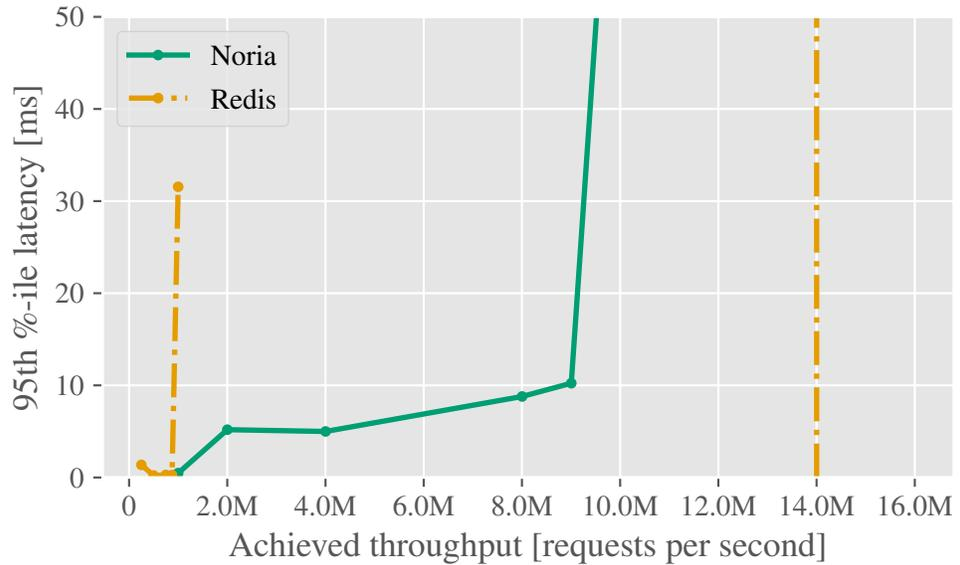
Figure 6.8.: Achieved throughput vs 95th %-ile request latency in cache-optimized vote. Offered load increases along the points on each line. The vertical line indicates  $16\times$  the highest Redis throughput, since Redis is single-threaded.
