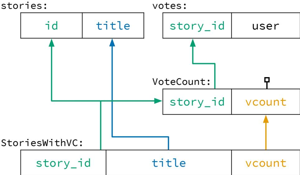
Figure 3.2.: Key provenance for each column in the `StoriesWithVC` view from Listing 2.1. Notice that `story_id` has multiple base table origins, and `vcount` does not trace back to any base table columns. The query only uses `story_id` as a parameter, so only its provenance is used to choose the upquery path.
