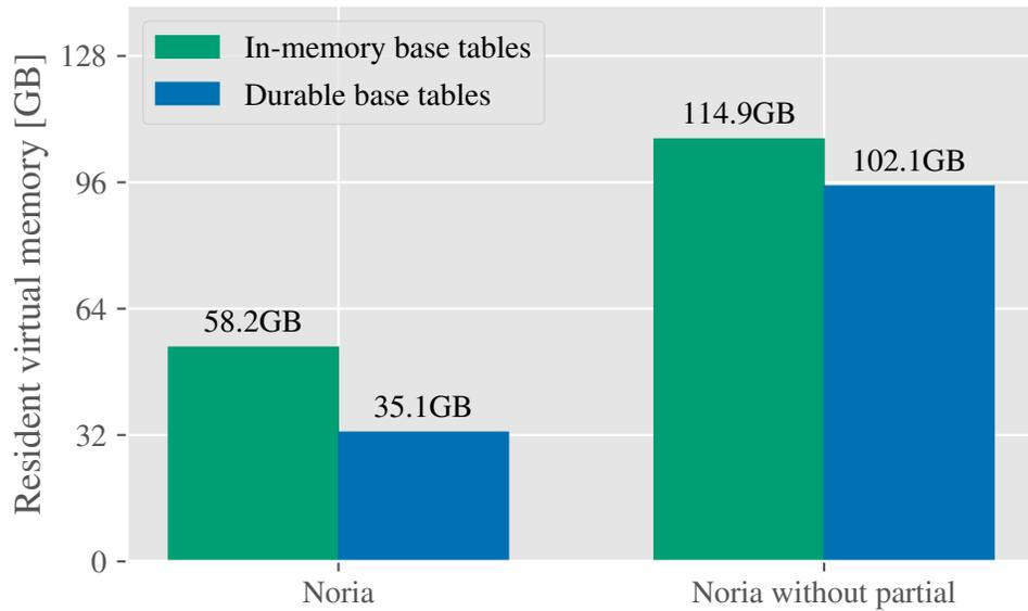
Figure 6.2.: Memory use two minutes into the Lobsters benchmark at 4.6k pages per second. Right bar in each pair show memory use when base tables are stored on disk using RocksDB.
