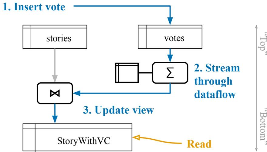
Figure 2.1.: Noria’s dataflow program to maintain Listing 2.1. Text describes the update path highlighted in blue. The dataflow inputs are considered the “top” of the dataflow, and the leaves are at the “bottom”. Parents are “upstream” of their “downstream” children.
