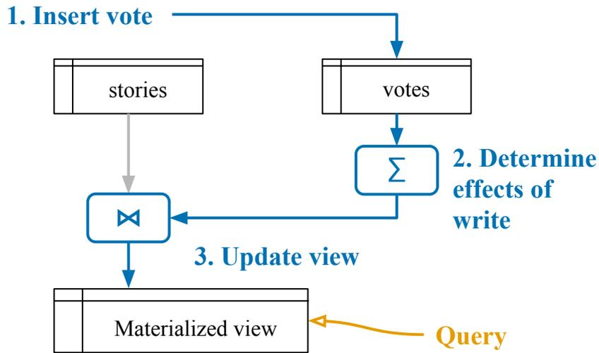
Figure 1.3.: Application query execution against a materialized view. Application queries only hit the view, which gives simple yet fast reads (**orange**). The database must determine the effects of every write and update the views to reflect changes (**blue**).
