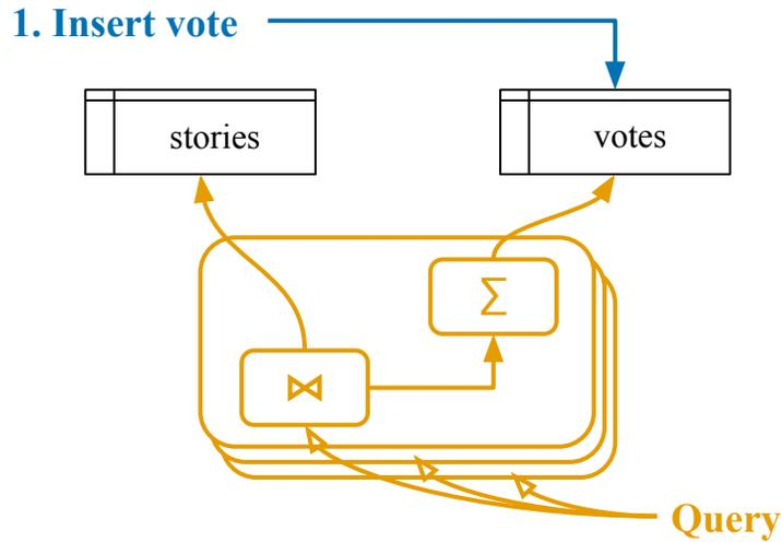
Figure 1.1.: Application query execution against a traditional database. Each application query runs in isolation, and may perform the same work (**orange**) repeatedly. Writes do little work (**blue**), even though they are less frequent in many applications.
