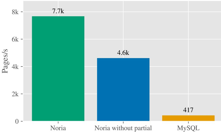
Figure 6.1.: Maximum achieved throughput on Lobsters benchmark with and without view materialization. Without view materialization, MySQL must compute query results each time. Traditional (full) view materialization runs out of memory at  $\approx 4.6k$  pages/second. Partial state allows Noria to reduce memory use significantly so that it can achieve higher throughput.
