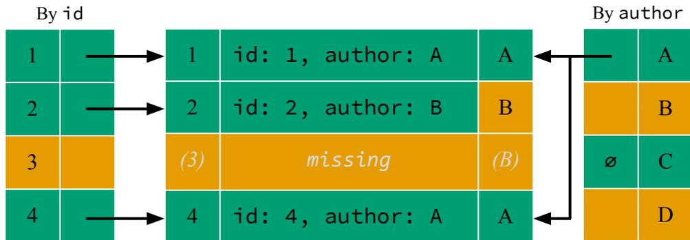
Figure 3.1.: Multiple indexes in a single view in Noria. Even though *some* rows for author B are **present**, some are **missing**, so the entry for B is missing in the **author** index. Even though there are no rows for author C, the index entry is not marked as missing, which would happen if Noria has already checked that there are indeed no rows in the base tables that match author C.
