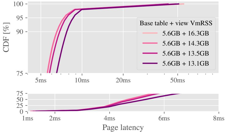
Figure 6.5.: CDF of sojourn latency in Lobsters at 1.5k pages per second as a function of eviction aggressiveness. The figure depicts steady-state operation—the benchmark has been allowed to run for two minutes before the latency is measured. Top figure uses a logarithmic x-scale to highlight the full range of the tail latency.
