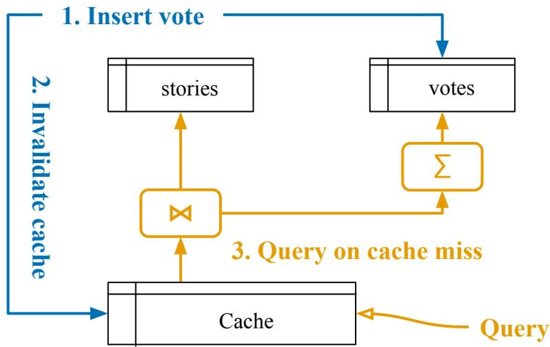
Figure 1.2.: Application query execution against a cache in front of a database. Application queries first check for cached results, and only execute database queries if the results are not cached. The application invalidates cached results so that later reads see the effects of new writes. The application logic for both reads (**orange**) and writes (**blue**) is more complex.
