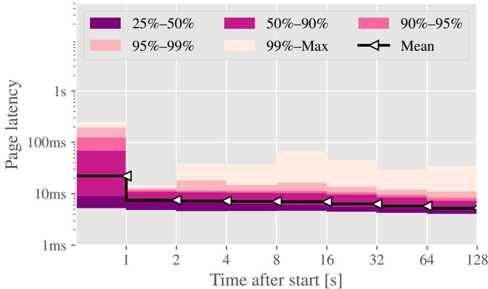
Figure 6.4.: Lobsters latency profile at 1.5k pages per second over time, starting when the first query is issued. Time increases along the x-axis, and each bin samples twice as long as the last. Later bins therefore capture more variance. The bin latency is plotted on a logarithmic scale. Lighter colors include more of the tail.
