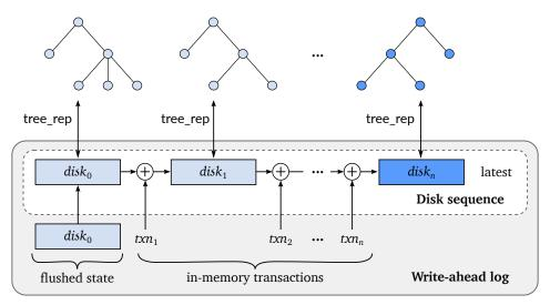
Figure 7-2: An illustration of FSCQ's disk-sequence abstraction
