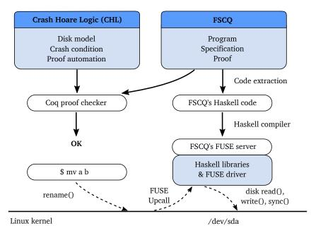
Figure 1-1: Overview of FSCQ's implementation. Shaded boxes denote source code written by hand. Solid lines denote processes. Dashed lines denote the call graph.
