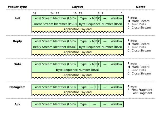
Figure 4-5: Stream data transfer packets
