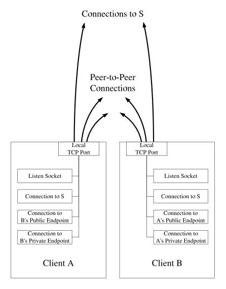
Figure 5-7: Sockets versus ports for TCP hole punching
