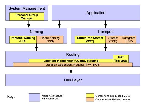
Figure 1-1: Architectural diagram of UIA and how it fits into the Internet architecture
