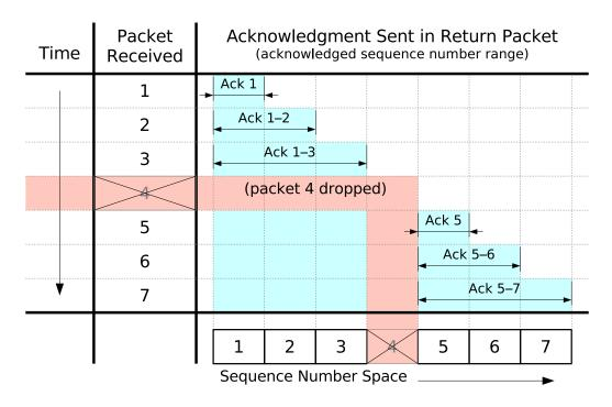
Figure 4-4: Packet acknowledgment example
