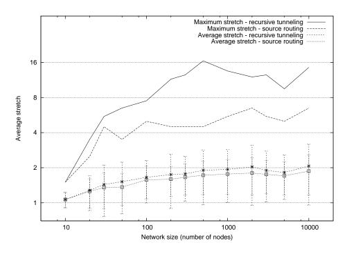
Figure 7-3: Network path stretch for source routing versus recursive tunneling
