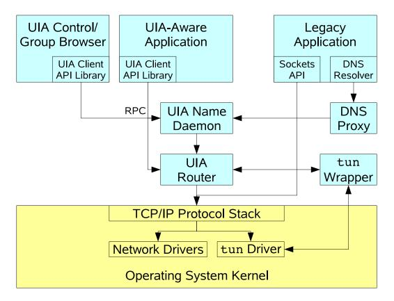
Figure 6-1: Structure of UIA prototype implementation
