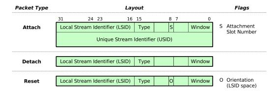
Figure 4-6: Stream control packets
