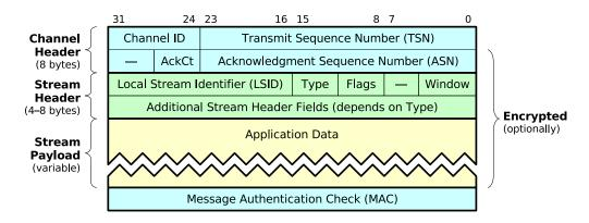
Figure 4-3: SST packet layout
