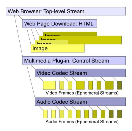
Figure 1-5: Example structured stream hierarchy in SST
