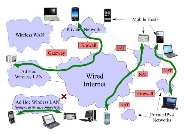
Figure 1-4: Global connectivity challenges for the UIA overlay routing layer
