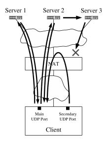
Figure 7-12: NAT check test method for UDP
