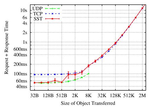
Figure 7-9: Transactional use of UDP, TCP, and SST over a  $2^{16} \times$  range of transaction sizes.
