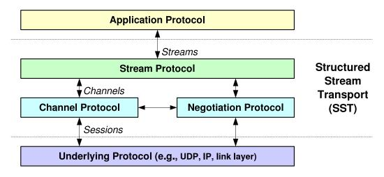
Figure 4-1: SST protocol architecture
