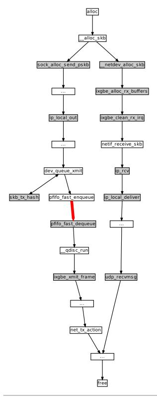
**Figure 2.** Partial data flow view for skbuff objects in memcached as reported by DProf. The thick line indicates a transition from one core to another. Darker boxes represent functions with high cache access latencies.
