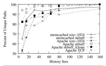
**Figure 4.** Percent of unique paths captured as a function of history sets collected. For all data types, the maximum number of unique paths is based on a profile with 720 history set. Only results for profiles with less than 160 sets are shown.
