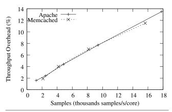
**Figure 3.** DProf overhead for different IBS sampling rates. The overhead is measured in percent connection throughput reduction for the Apache and memcached applications.
