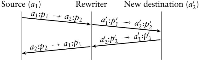
FIGURE 4—Action of a generic NAT with port translation. Each arrow represents a packet with the given flow ID.
