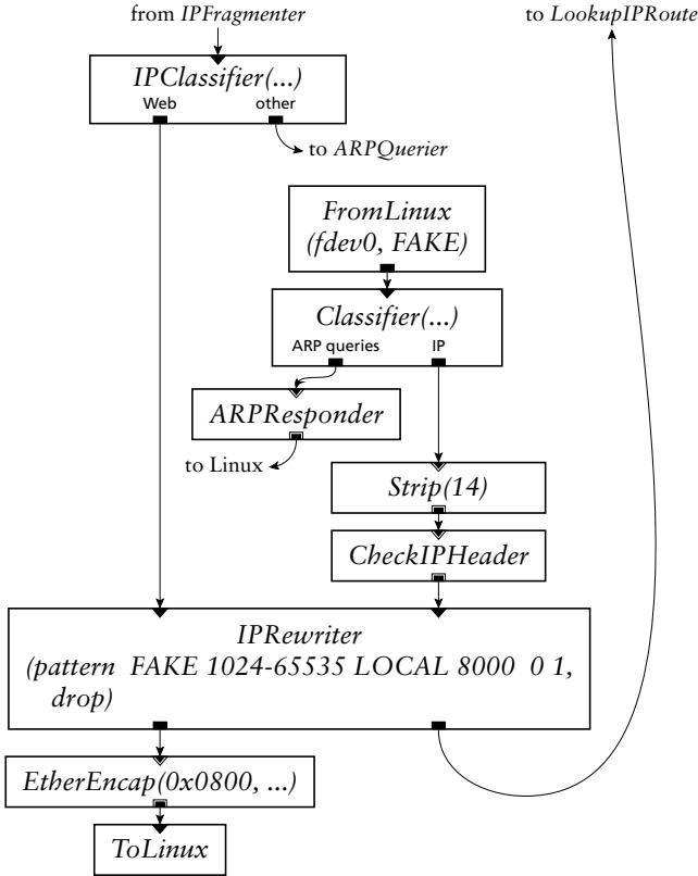
FIGURE 8—A transparent Web traffic diverter extension for the IP router configuration.
