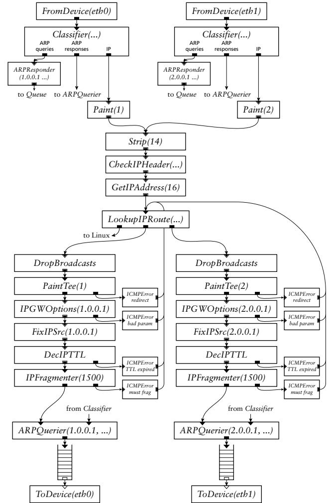
FIGURE 3—An IP router configuration.
