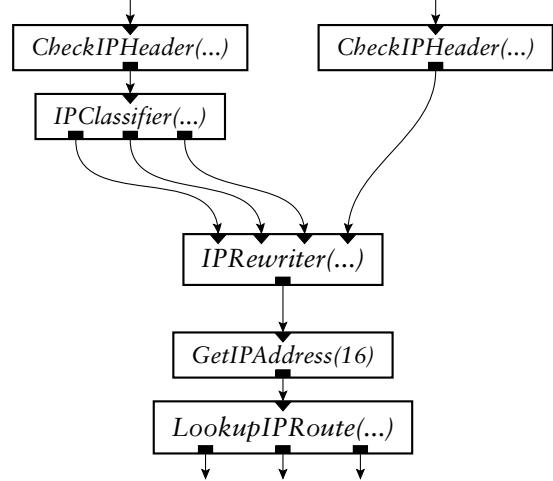
FIGURE 7—A router configuration for port routing.
