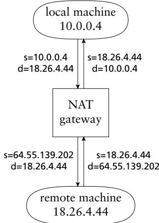
FIGURE 1—Basic NAT, as described in RFC 1631 [5]. The local machine has a private IP address. When it sends packets to an Internet host, the NAT gateway assigns it an address from a public address pool and rewrites the packets accordingly. Replies are rewritten to use the original private IP address.
