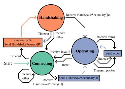
Figure 5-3: FakeWire Handshake Process
