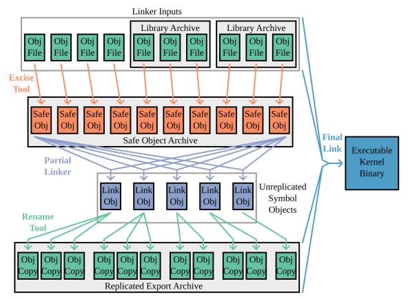
Figure 4-5: Overview of the Replication Linking Process
