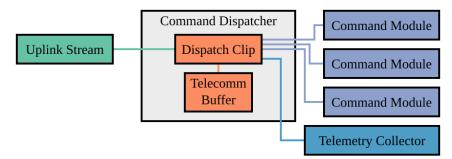
Figure 6-10: Command Dispatcher Structure
