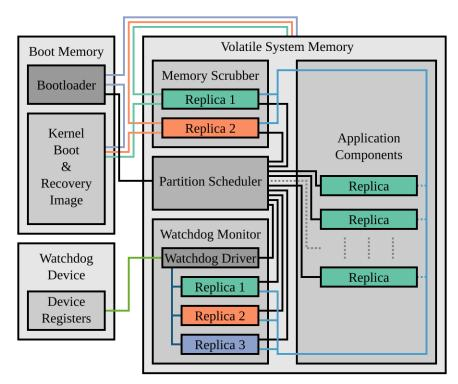
Figure 3-2: A diagram of the kernel components present during runtime.
