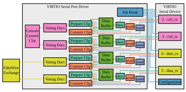
Figure 6-2: VIRTIO Driver Structure
