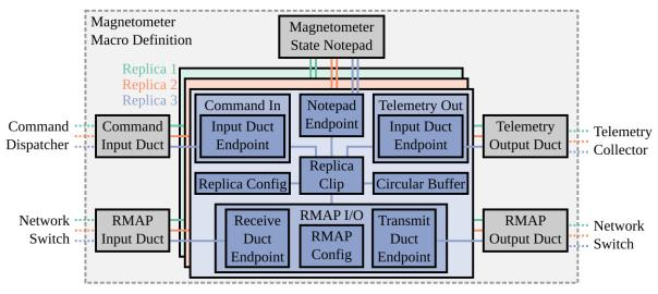
Figure 3-6: Example Replicated Magnetometer Component
