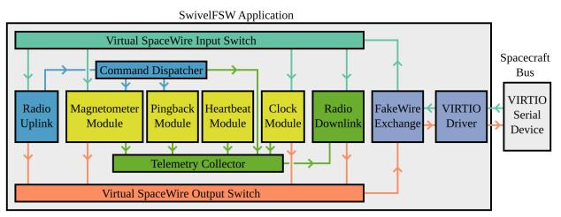
Figure 6-1: Overview for the SwivelFSW Flight Software
