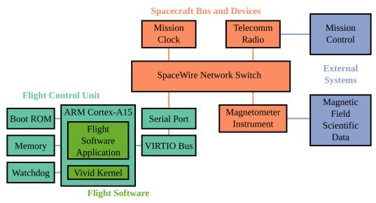
Figure 5-1: Testbench Spacecraft Avionics
