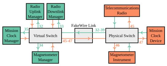
Figure 6-6: Complete SpaceWire Network Map
