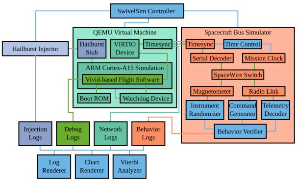
Figure 7-1: SwivelSim Simulation Overview
