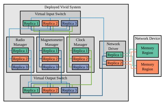
Figure 3-1: A simplified diagram of flight control software implemented using Vivid
