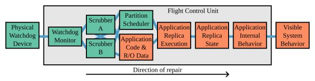
Figure 3-9: Vivid's sequence of repair
