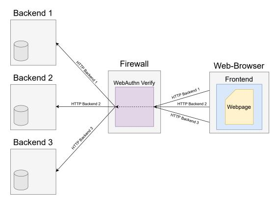
Figure 4-5: A WebAuthn firewall handles multiple backend targets for a single frontend.
