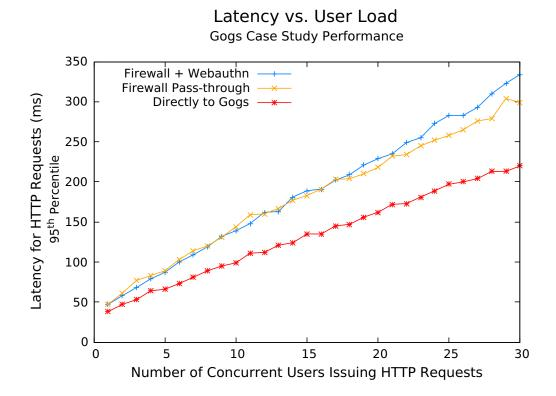
Figure 7-3: The 95<sup>th</sup> percentile run times of three different Gogs setups under load. The x-axis is the number of users issuing requests concurrently, and the y-axis is the run time latency in milliseconds. The three experiments are: using Guarda with WebAuthn enabled, using Guarda with WebAuthn disabled, issuing requests directly to the Gogs server without WebAuthn transaction authentication. There is a latency penalty to using the WebAuthn firewall.
