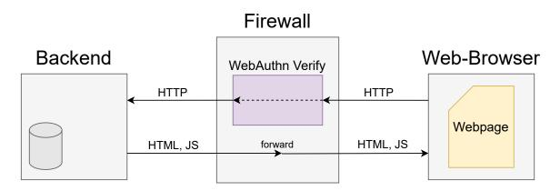
Figure 4-4: The positioning and role of the WebAuthn firewall in a server-side rendering paradigm web service.
