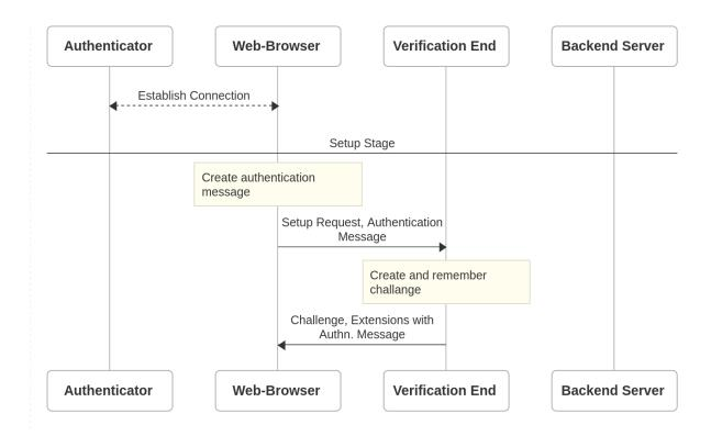
Figure 3-3: The flow of events during the setup stage of WebAuthn transaction authentication.
