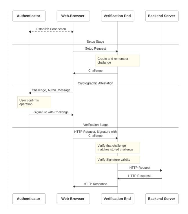
Figure 3-1: A simplified overview of the flow of events during WebAuthn transaction authentication, subdivided into three stages.
