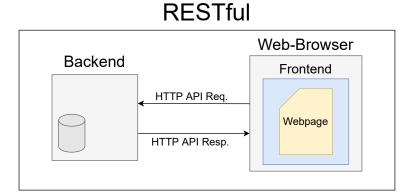
Figure 1-3: The architecture design of a RESTful web application.
