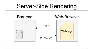
Figure 1-4: The architecture design of a server-side rendering web application.
