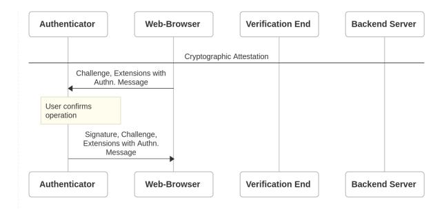
Figure 3-4: The flow of events during the cryptographic attestation stage of Web-Authn transaction authentication.
