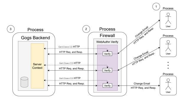
Figure 7-2: The experiment setup to measure the performance overhead of Guarda under load.
