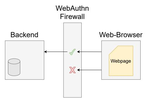
Figure 1-2: Basic depiction of the WebAuthn firewall functionality.
