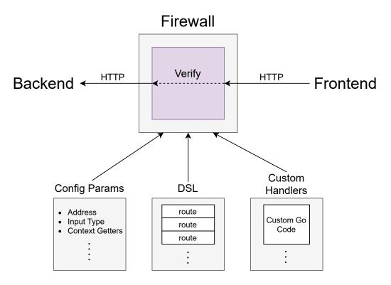
Figure 4-2: The functionality of the WebAuthn firewall fully depends on the configurable components passed into it.
