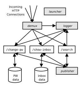
**Figure 1**: Block diagram of the OKWS system. Standard processes are shaded, while site-specific services and databases are shown in white. The privileged *launcher* process launches the *demux*, *publisher*, *logger* and the site-specific services. The databases shown might either be running locally, or on different machines.
