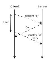
**2. [10 points]:** Show a scenario in which the server gives lock "a" to two different clients, violating the goal that only one client should have the lock at any time. (Draw a message time diagram.)
