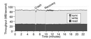
Figure 15: A brick fails then recovers in a 22-brick FAB cluster running the 3-way quorum-based replication protocol under the DB workload. FAB can mask the failure without causing any I/O errors.
