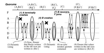
Figure 8: Reconfiguration example. This seggroup initially replicates data on bricks A,B,C, with witnesses D,E participating only in view transition. At the top, the set of active quorums formed at each moment is shown. After A and B crash, C is still able to form a singleton view with help from the witnesses. After B recovers and F is added, they ensure that they store values written to the seggroup before removing the old view  $\{C\}$ .
