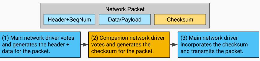
On error, either A) the packet will have an invalid checksum, and get rejected by the destination device, or B) the same packet will be sent, but the re-used sequence number will let it be rejected.
