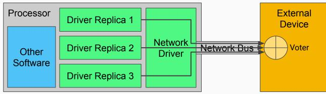
• This works if the device is **specially designed** for the spacecraft, and if enough **network capacity** is available to triplicate the messages.
