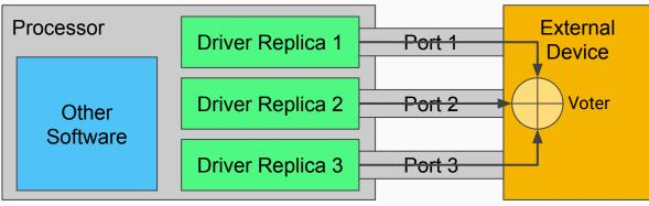
• This works if the device is **specially designed** for the spacecraft, and it **directly connects** to the processor. But many devices don't qualify.
