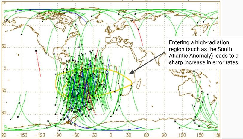
SOURCE: R. DeCoursey, R. Melton, and R. Estes, "Non radiation hardened microprocessors in space-based remote sensing systems", Proc. SPIE Sensors, Systems, and Next-Generation Satellites, vol. 6361, 2006.
