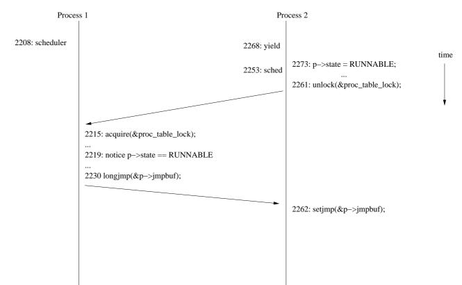
In this scenarib, the scheduler longjmps to the buffer before the process has initialized it with setjmp. Thus the re-started process will be running with a stale register set, i.e. with an incorrect stack pointer.
