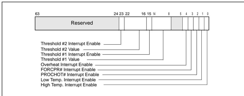
Figure 13-10. IA32\_THERM\_INTERRUPT Register
