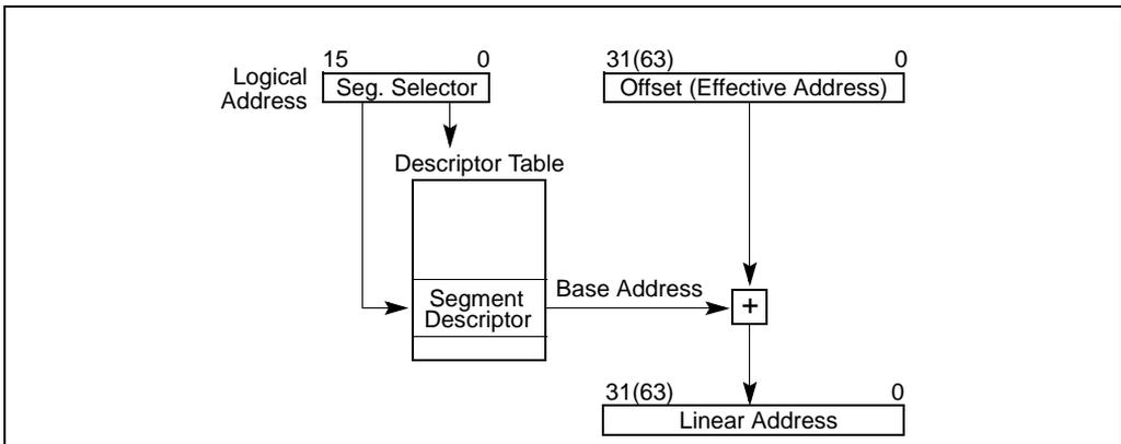
**Figure 3-5. Logical Address to Linear Address Translation**
