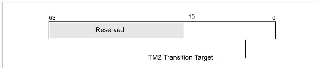
Figure 13-5. MSR\_THERM2\_CTL Register for Supporting TM2
