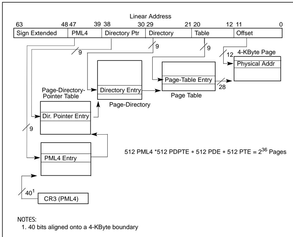
Figure 3-24. IA-32e Mode Paging Structures (4-KByte Pages)
