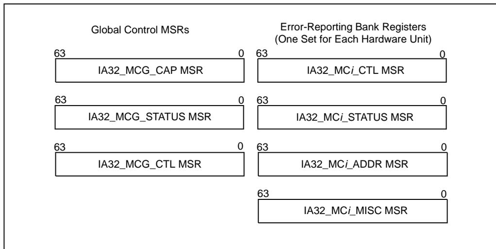
Figure 14-1. Machine-Check MSRs
