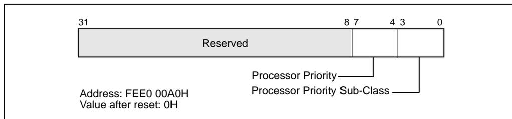
**Figure 8-19. Processor Priority Register (PPR)**
