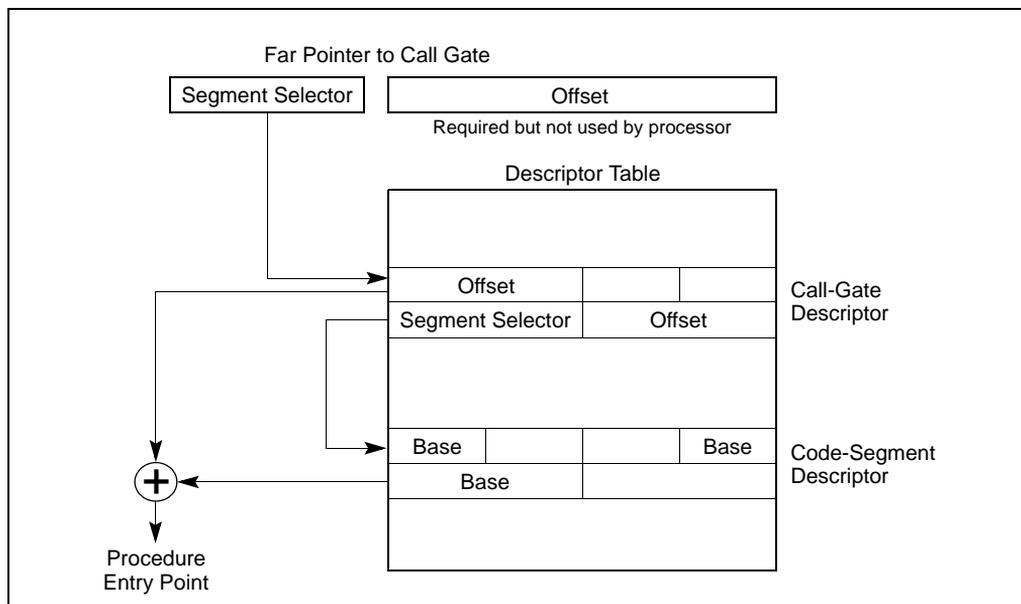
Figure 4-10. Call-Gate Mechanism
