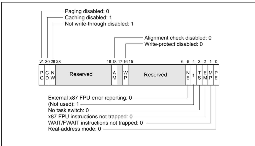
Figure 9-1. Contents of CR0 Register after Reset
