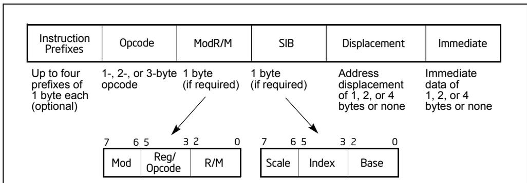
Figure 2-1. Intel 64 and IA-32 Architecture Instruction Format
