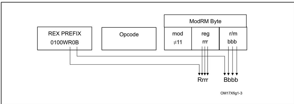
**Figure 2-4. Memory Addressing Without an SIB Byte; REX.X Not Used**
