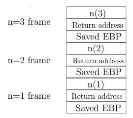
Figure 4.16: Stack frames for factorial function
