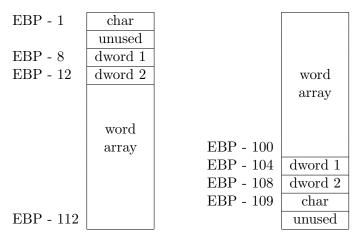
Figure 5.2: Arrangments of the stack
