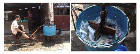
Figure 2: MayaPedal's prototype washing machine shows that demand exists, but it is difficult to use and it damages clothing.
