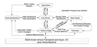
Fig. 8. Tapestry implementation. Tapestry is implemented in Java as a series of independently scheduled stages (shown here as bubbles) that interact by passing events to one another.
