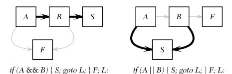
(Any basic block with two branches has, as its final action, a test to see if it some expression is zero: one branch is taken on zero, the other if not. In the figure, thick black arrows represent the nonzero branch and thin grey arrows represent the zero branch.) *Prolacc* will apply either transformation only if *B* cannot generate any state code and *B* has not been outlined relative to *A*.
