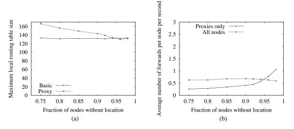
**Figure 7**: (a) Location proxies slightly increase the maximum route table size, which is measured across all nodes for the entire simulation. (b) Location proxies do more work and handle a larger percentage of traffic when fewer nodes know their location.
