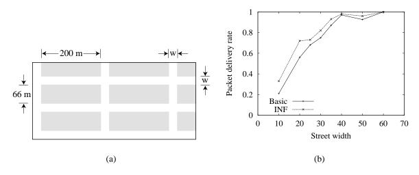
**Figure 9**: Intermediate node forwarding (INF) improves packet delivery in urban scenarios. (a) shows the urban scenario used in simulation. Nodes can only move in the streets (white), avoiding the city blocks (gray rectangles). Packet transmissions cannot travel through city blocks. (b) shows INF's improvement in forwarding rate over the basic routing protocol.
