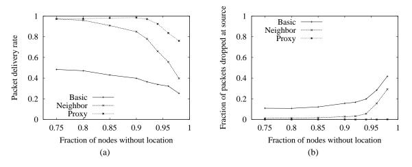
**Figure 6**: (a) The location proxy technique delivers more packets. Proxies make geographic forwarding useful when as many as 95% of nodes do not know their location. (b) All nodes find proxies. No packets are dropped at the source using the proxy technique, implying that every node manages to find a proxy.
