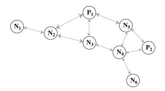
**Figure 3**: Packets need not travel out of the way to go through proxies. In this example with a two hop DSDV radius,  $N_1$  is sending to  $N_6$ ; their proxies are  $P_1$  and  $P_2$ , respectively. Because of the proxy route propagation rules,  $N_2$  has an explicit route to  $P_2$ , via  $N_3$ . Therefore packets will travel from  $N_1$  to  $N_3$ , bound for  $N_6$ 's proxy. But  $N_3$  has an explicit route to  $N_6$ , and the packets avoid both  $P_1$  and  $P_2$ .
