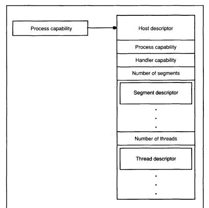
Figure 4. Layout of a process descriptor.
