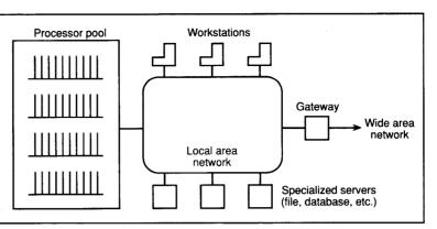
Figure 1. Four components of the Amoeba architecture.
